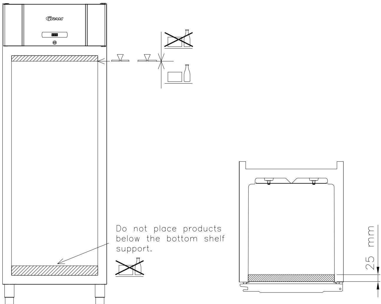
All products to be stored, that are not wrapped or packed, must be covered in order to avoid unnecessary corrosion of the inner parts of the cabinet.
